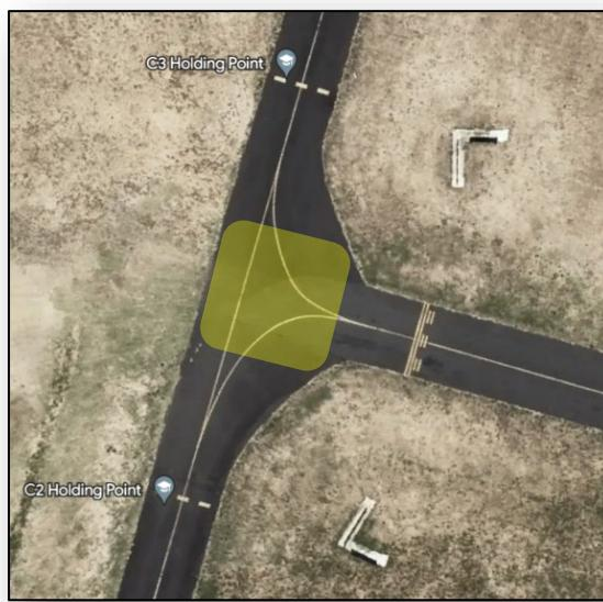
This stop should also be used to confirm that the brakes are operating effectively prior to taxiing into the Waikato Aviation apron area. If you stop on the grass in winter, you may require additional power to get moving again and the brake check might not be as effective than stopping on the sealed taxiway.
