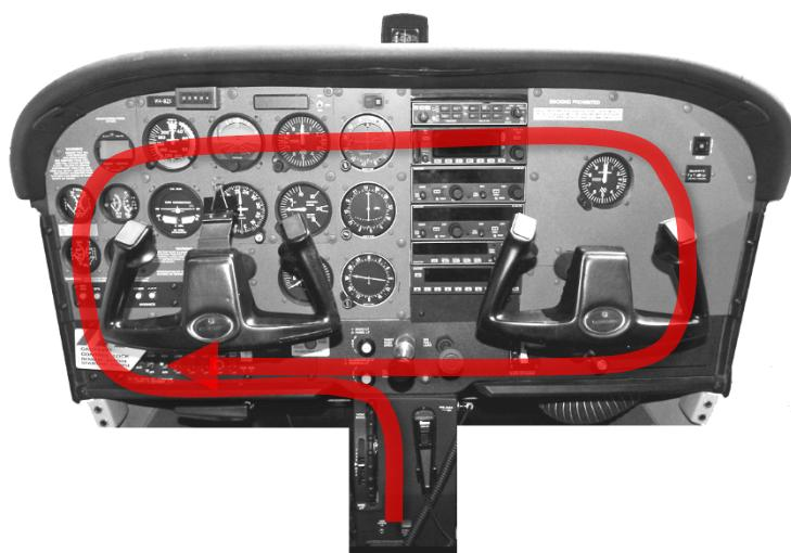
Starting between the seats, carry out first an **electrical power off check** of the engine and instrument systems as per the diagramme above →. During the first flight of the day, exercise the mixture, throttle, ventilation/cabin heating levers as well as the alternate static vent.
