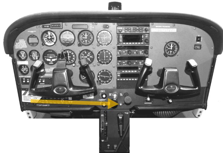
Once the flow check is complete the battery (and alternator) shall be turned on, lights selected on as required and the engine primed for start see flow above.
